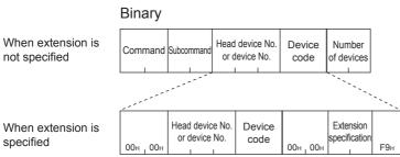
The following shows the module access device and request data.
