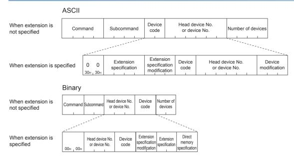
The following shows the approach for devices, index registers, long index registers and request data.
